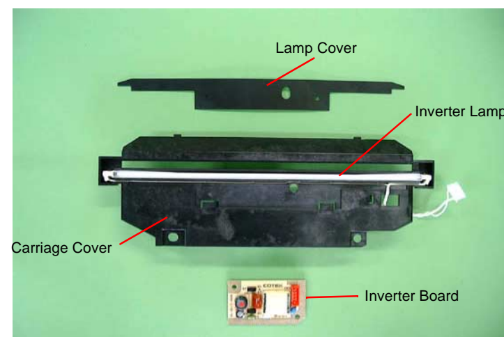
Figure 4-12. Inverter Lamp Removal (2)
