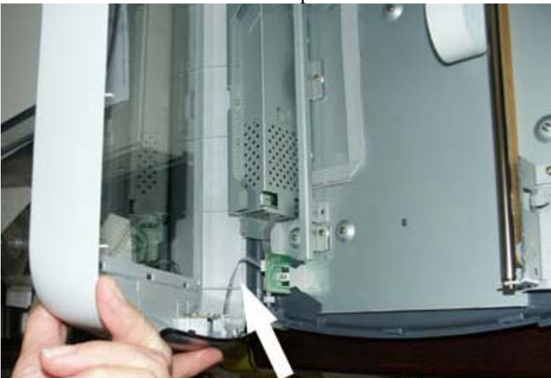
Picture 4: This picture shows the wire, and connector, referenced in step 6.
