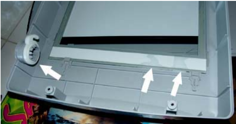
Picture 7: White calibration strip. Each time you scan (or turn the scanner on, not sure which), the scanner 'scans' this strip to determine what 'white' is. As indicated by the rightmost two arrows, cleaning liquid got behind the glass, and discolored the strip.
