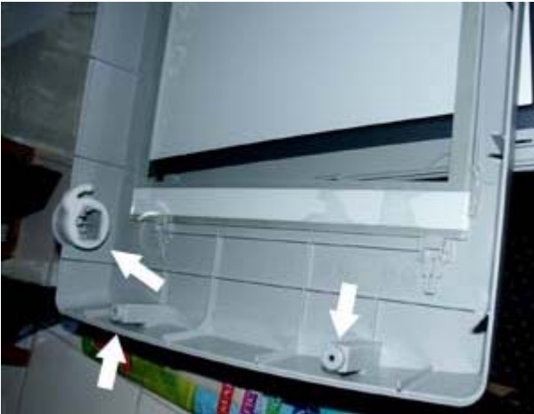
Picture 2: Scanner locking mechanism (far left of picture) in the upper frame that interferes with the pin shown in picture 1 (also shows the two screw holes that attach top to bottom). See also picture 7.
